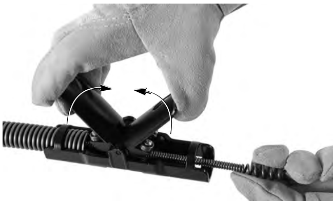
Figure 5 – Feeding Cable Through AUTOFEED® Assembly
