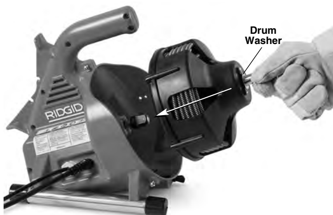
Figure 16 – Inserting Drum Into Machine
